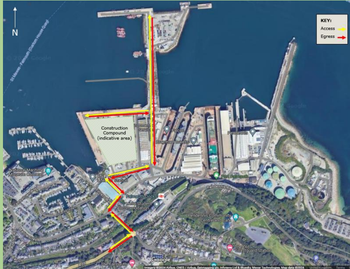
Site Access and Egress Throughout Demolition and Construction Stage
